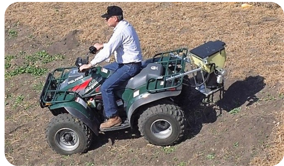
Seed slinger products such as these pictured from Truax Company, Inc. can be hand cranked or mounted to an ATV for broadcast seeding larger sites (photo credit:
